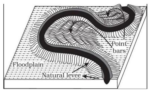
Fig 11 : Natural levee and point bars
